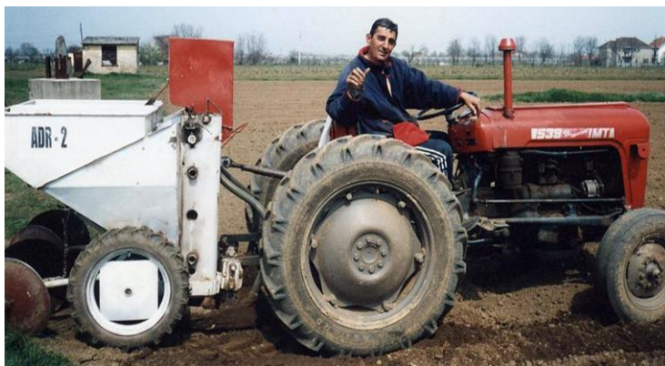
Figure 1. Two-row automatic potato planter with fertilizer dispenser
